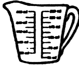
LIQUID MEASURE Most common size is 250mL Smallest amount on measure is 50mL Has division lines every 10mL or 25 mL
